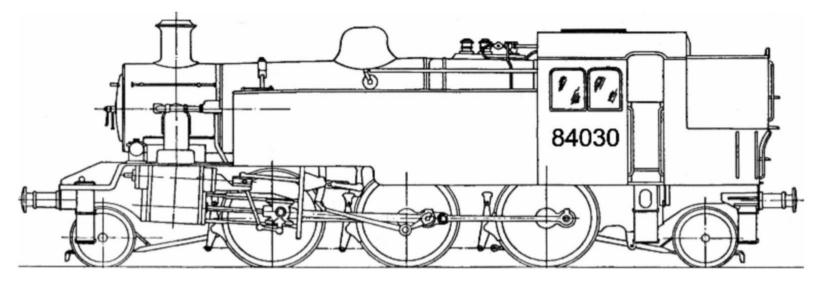
Principal Characteristics:Length - 38' 9<sup>1</sup>/<sub>2</sub>"Height - 12' 9<sup>1</sup>/<sub>2</sub>"Width - 8' 7<sup>1</sup>/<sub>2</sub>"Water capacity - 1350 gallonsCoal capacity - 3 tonsWeight - 66 tons 5 cwt
