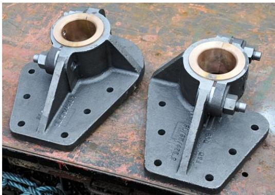
Brake Shaft Bearings (prior to finishing the studs)
