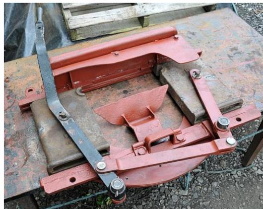
Fire-Door assembly nearing completion.
