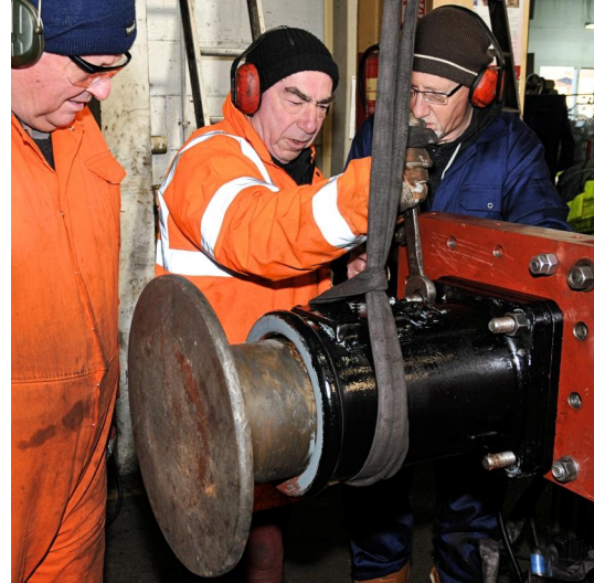
Trial fitting the front buffers
