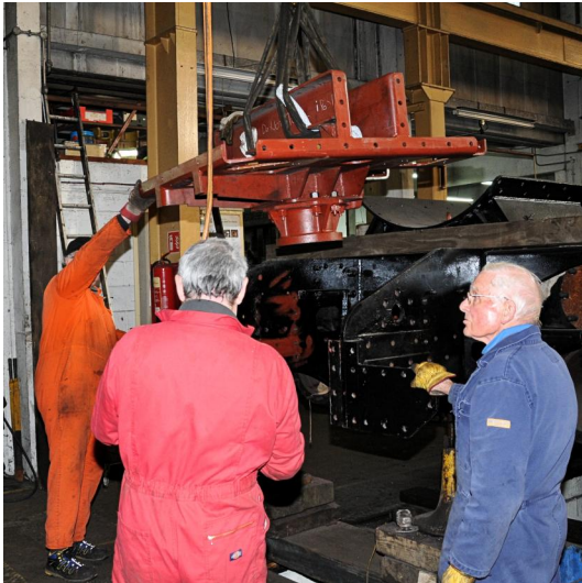
Lifting in the front box complete with truck centre
