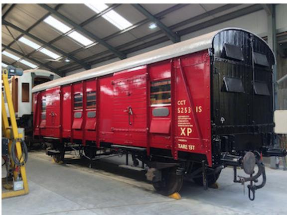
In comparison, **No. 2531**, the Camelot Locomotive Society's Lancing-built Covered Carriage Truck (CCT) of 1955, represents the final design of that SR van family. After completion of the major body overhaul earlier in the year, in October it was able to go on the lifting jacks and receive its mechanical overhaul. At the same time, the remaining steelwork on the underside of the van was cleaned up and repainted. It is now all but
