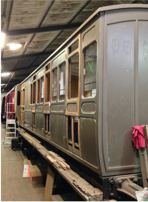
The two LB&SCR Stroudley carriages in the works continue to make progress. **Brake Third No.949** now has all its glazing in the passenger area, all but one of its doors overhauled and hung, and a start made on panelling these. Excepting internal quarterlight (window) frames and the unique Stroudley patent communication system, the interior is essentially complete.
