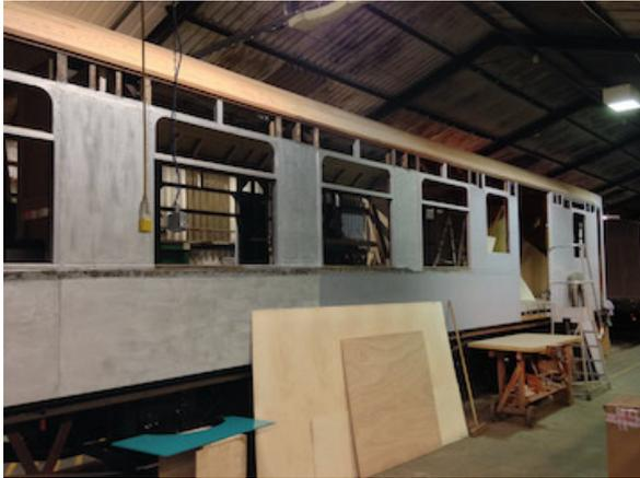
The huge quantity of work undertaken on Car 54 is far beyond the scope of this article, but suffice to say that the structural element of the rebuild is essentially now complete, the (new) gangways and (replacement) buffers coming together, the wiring well-advanced, the overhaul of the marquetry and manufacture and trimming of the new seats well in hand, and the internal ceilings going up. The photos, taken on 14 Dec., 2019, show
