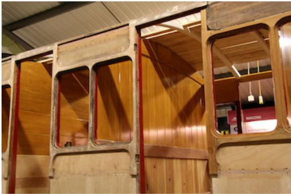
**Stroudley Full Third No.328** has had its external panelling fitted, and the decoration of the partitions completed prior to fitting the roof, the timbers for which are in an advanced stage of preparation. Work has re-started on the doors.
