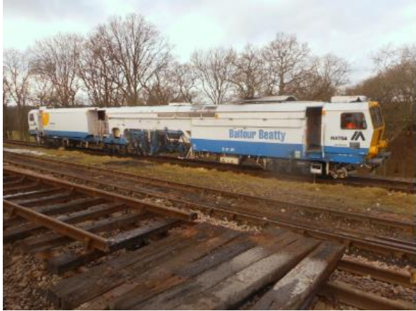
Balfour Beatty main line tamper with trainees on board on its way to Sloop Bridge.
