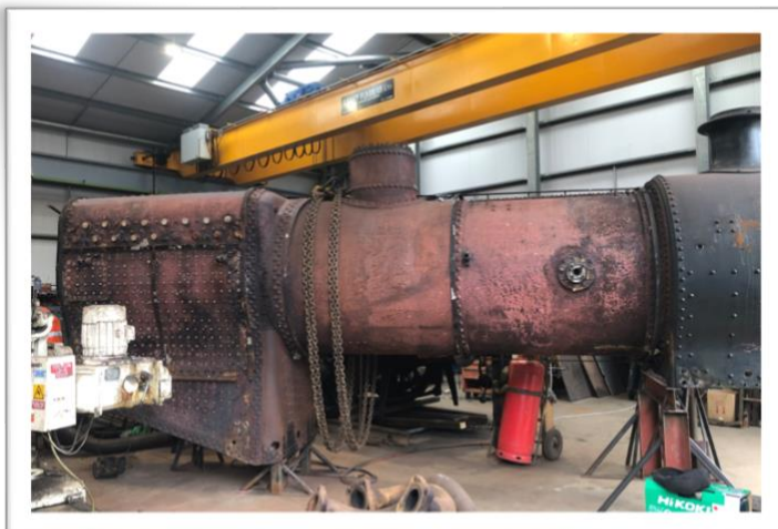
Left: The boiler out of the frames ready for needlegunning
