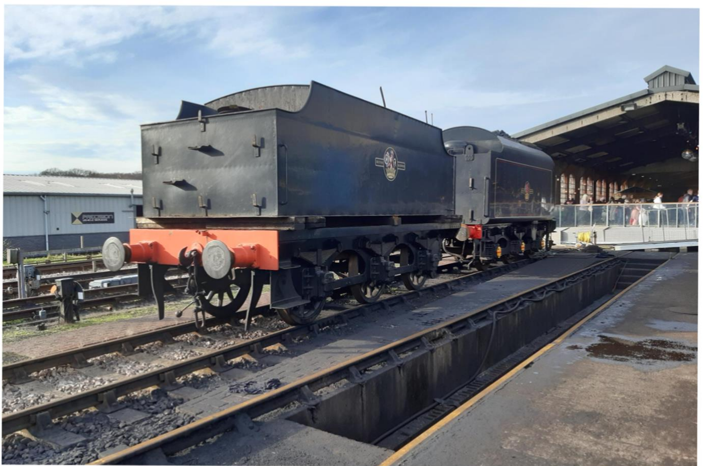
Above: 541's tender tank freed up and raised off the tender chassis, awaiting removal.
