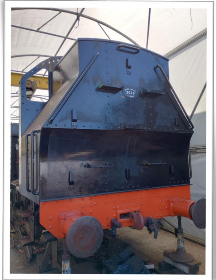
Above: Bunker with all lamp brackets and steps plus a coat of paint to the bunker back panel and buffer beam
