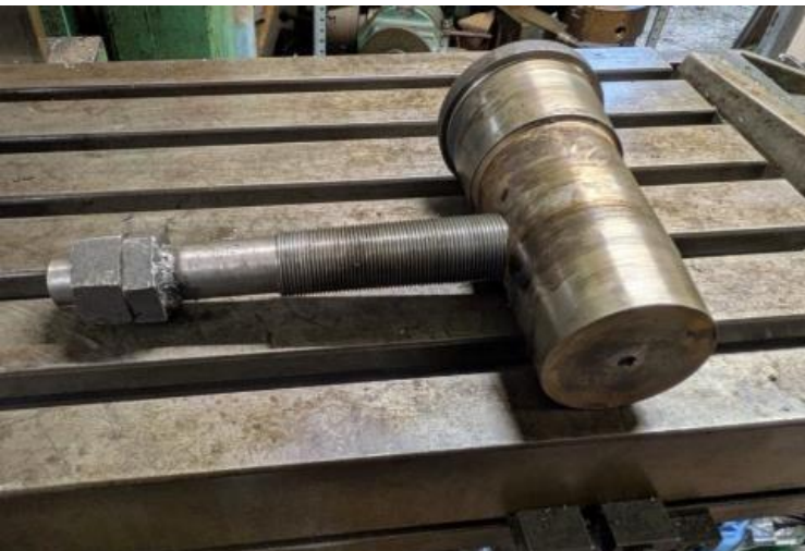
Fig 12. The dummy gudgeon pin with the fine pitched screw used to apply pressure onto the piston rod.
