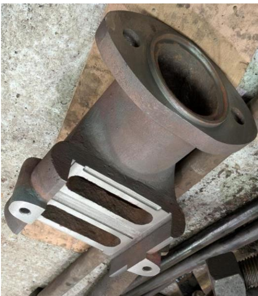
Fig 15. Here is the re-machined regulator body. When will this be installed!
