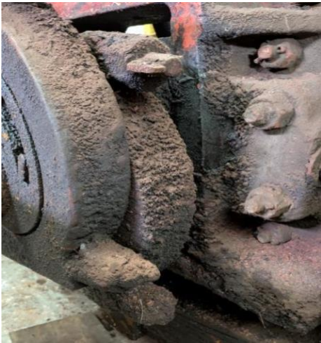
Fig 4. This shows the two right hand eccentric straps with the horn behind that is bolted to the frames.
