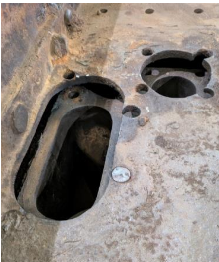
Fig 3. the plate over laying the valve chests. The cut off stud near the front shows the problem. These studs are firmly rusted into their threaded holes.
