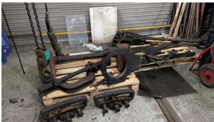
Fig 9. Valve gear parts removed, in the foreground the expansion links, the omega shaped part is an intermediate valve rod that dodges over the leading axle, and eccentric straps and rods behind.
