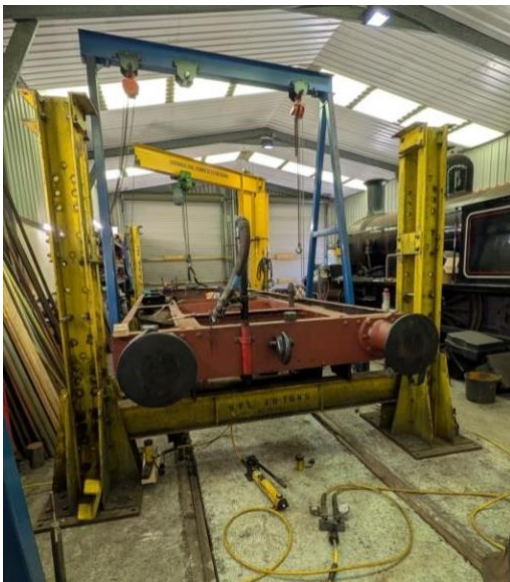
Fig 4. This shows the two right hand eccentric straps with the horn behind that is bolted to the frames.
