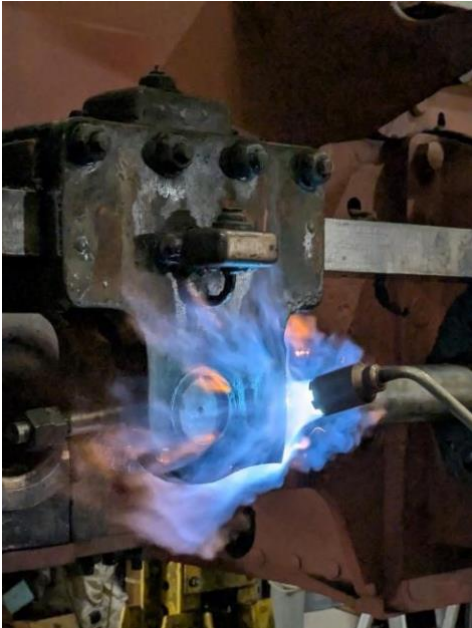
Fig 13. The crosshead here is being heated to expand it while force was being applied to the piston rod.
