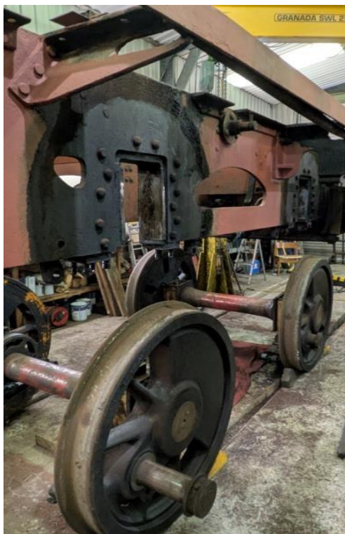
Fig 8. The frames now lifted, the wheels still on the rails. Note the dirt behind the area previously made inaccessible by the wheels.
