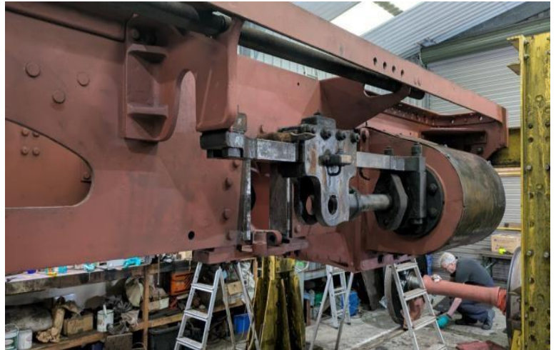
Fig 5. The frames now cleaned, needle gunned and in primer.
