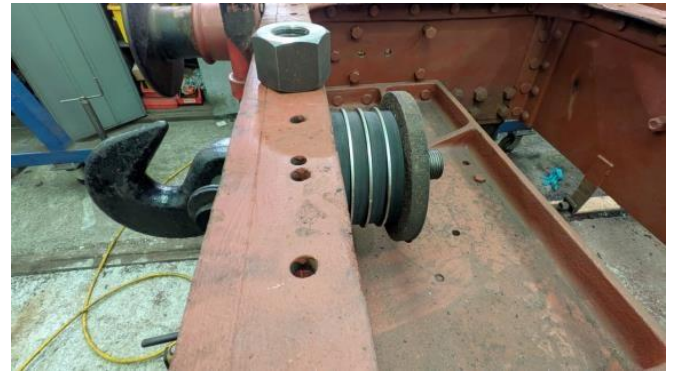
Fig 2. Reworked coupling hook being trial fitted. The new nut can be seen on top of the framing
