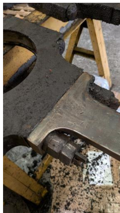
Fig 9. Valve gear parts removed, in the foreground the expansion links, the omega shaped part is an intermediate valve rod that dodges over the leading axle, and eccentric straps and rods behind.
