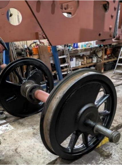
Fig 11. The cleaned wheels in black undercoat.
