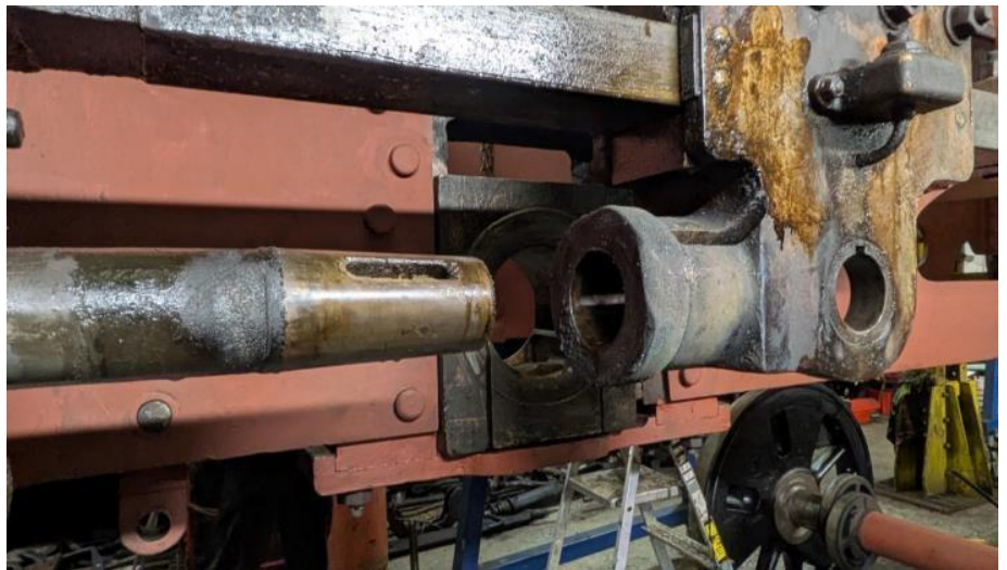
Fig 14. Here you can see the taper on the piston rod that fits into a matching one in the crosshead. Also the slots in both items that take the key that retain the parts in case of shock loadings such as water trapped in the cylinders.
