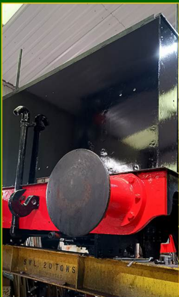
Wasted tank section cut out waiting for a replacement plate to be welded in.
