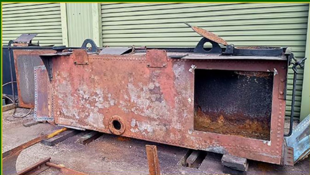
Wasted tank section cut out waiting for a replacement plate to be welded in.
