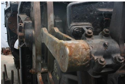
Trial Fitting of Reversing Gear
