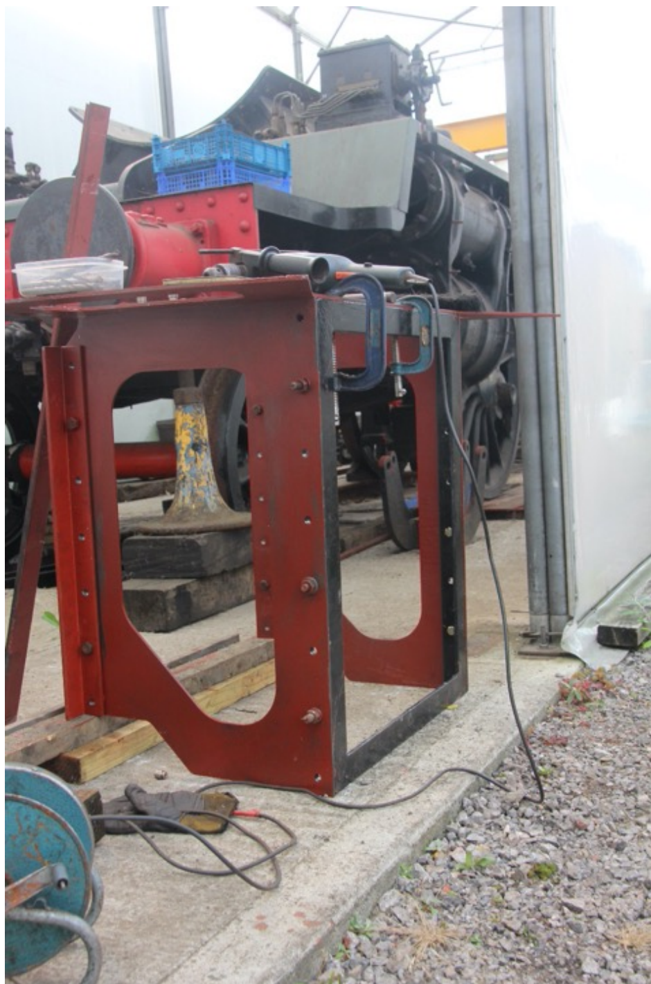
Start of the shovelling plate assembly
