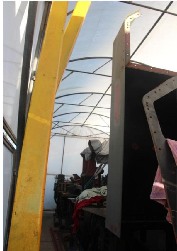
Now that the shelf is in position the next planned action is to bolt on the top section panel. Whilst all this work has been going on Harry has been going around with his paint pot in an attempt to stop rust breaking out especially around drilled holes, bolts and rivets.
