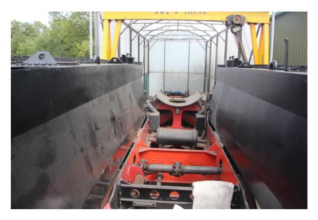
Thanks must be given to Ben and his workshop team in the supervising and positioning of the tanks onto the frame of 84030.
