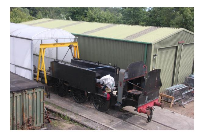
To transport the tanks a HIAB lorry capable of lifting 5 tonnes with a 15-metre reach was arranged, the plan being for the tanks to be lifted straight onto the frame and with the HIAD pulled up on the tramway adjacent to the frame it was well within its reach.
