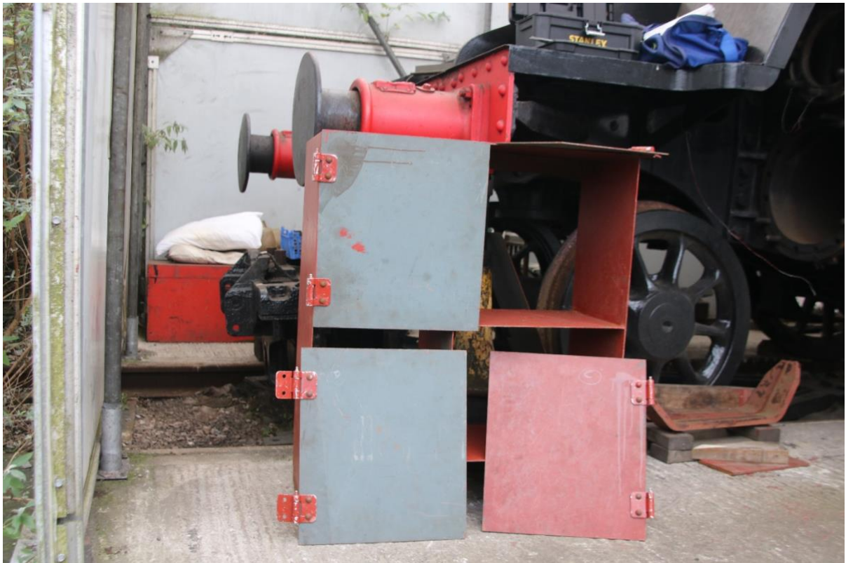
Tool Box under construction with one door fitted
