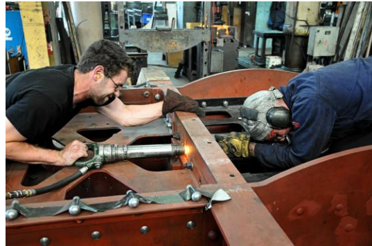
Hot riveting nearing completion
