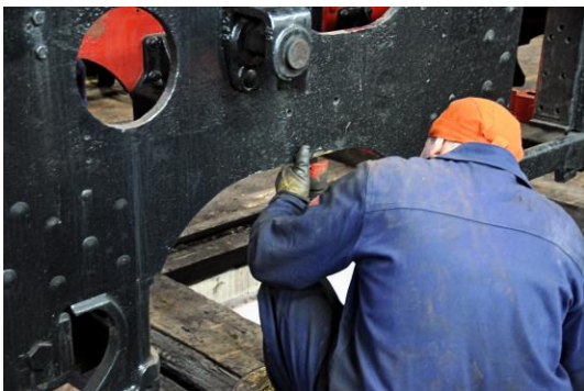
Setting the frames on stands
