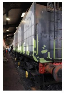
With much elbow grease all running plate bolts have been loosened greased and placed back. This will aid the amount of time needed in the works to remove the cladding.
