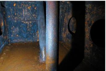
Lastly concerning the tender the coal space has been completely cleaned out and is now ready for wirebrushing then the first coat of protective paint.
