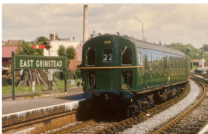
Class 207 DEMU in British Railways Livery with Orange Hand Rails and Buffer Beam at East Grinstead High Level Station
