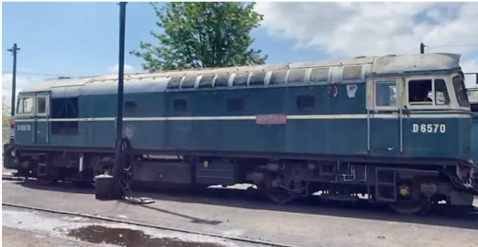
*The locomotive is in good mechanical condition and has been stored undercover out of use for several years at the Kent and East Sussex Railway. On arrival at the Bluebell Railway, it will not enter service immediately, however the new owners will implement a re-commissioning programme to ensure the locomotive is reliable before being available for service and at the same time undertake a number of bodywork and roofing repairs to make the loco weathertight.*
