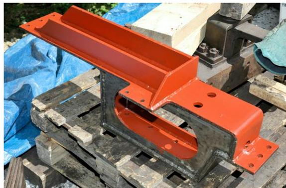
Reversing Gear Bracket Being Restored
