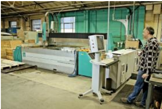
The water jet machine profiling the first frame plate.
