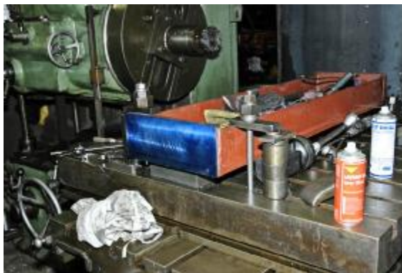
The first stretcher with frame flanges machined.
