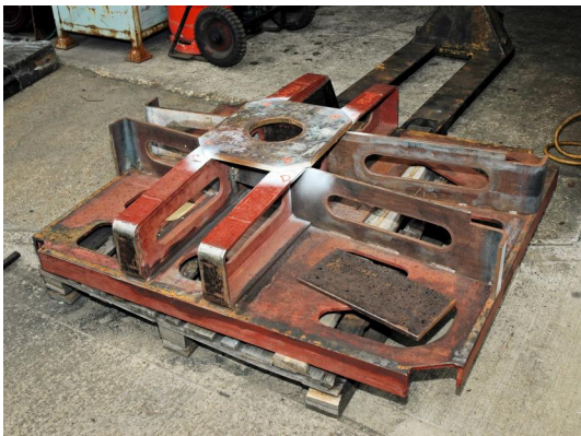
Hind drag-box ready for welding
