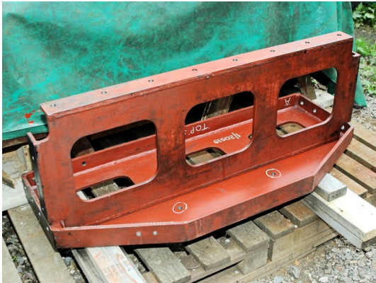
Trial assembly of the two stretchers to rear of firebox
