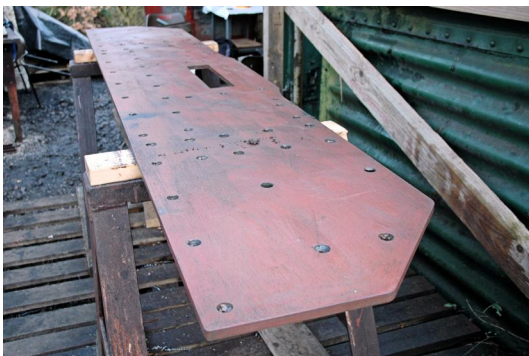
The hind buffer beam ready for assembly
