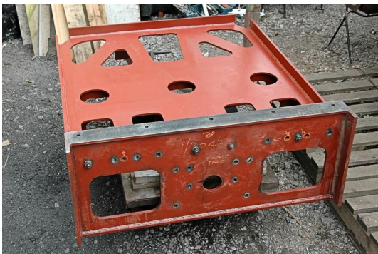
Drag-box and vertical stretcher drilled
