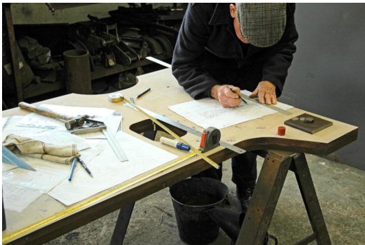
Marking out the frame extension plates
