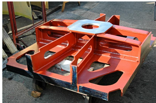
The hind drag-box after machining
