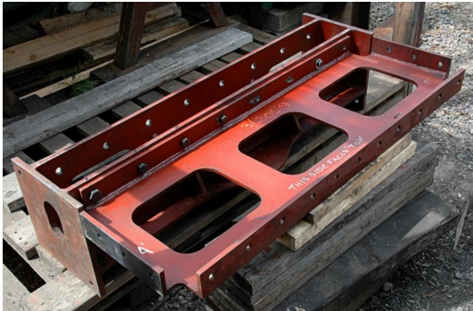
Horizontal stretcher to rear of firebox and brake cylinder support stretcher
