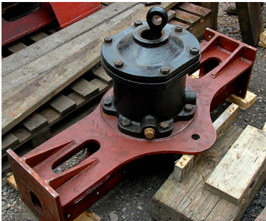
Brake cylinder fitted to support stretcher
