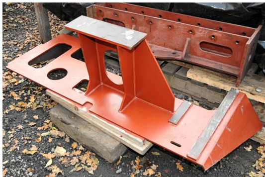
LHS rear tank support and reversing gear mounting
