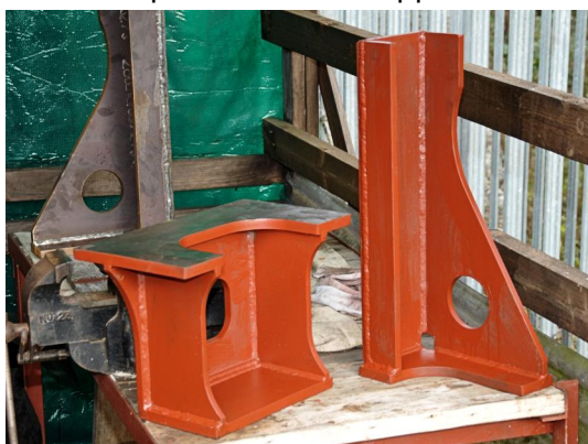
Boiler steady support and front tank support brackets
