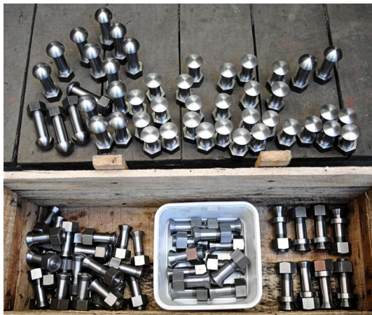
Fitted bolts and nuts for the frame extension
