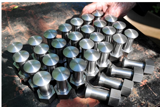
More fitted bolts and nuts for the frame extension
