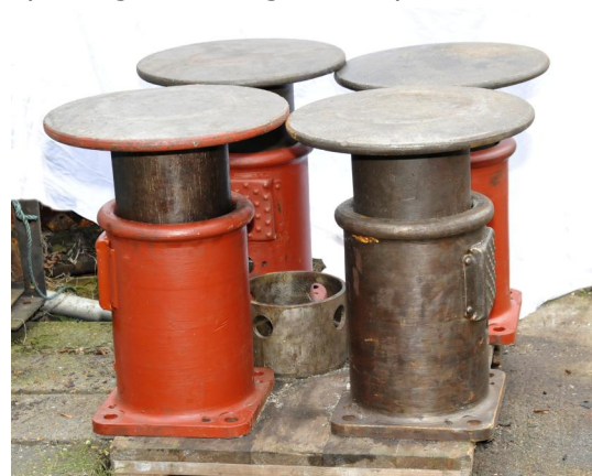
Set of partly restored buffers for 84030
