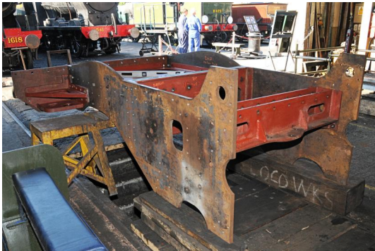
Trial assembly of rear frame extension
