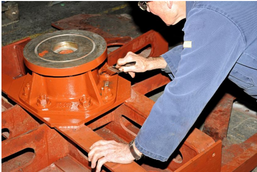
Primer being applied to the hind truck centre
