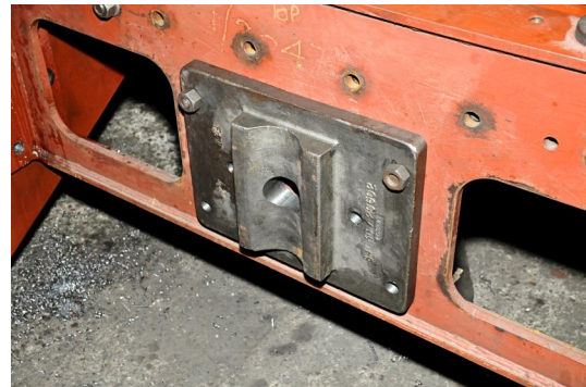
The rear draw-gear pivot plate in position
