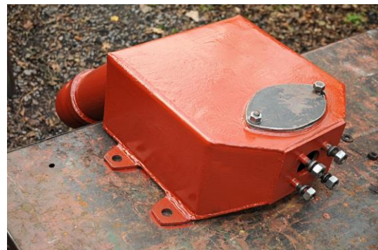
Front sandbox complete with new access cover
