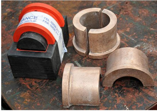
Pattern set and castings for the brake shaft bearings
