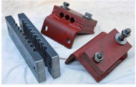
Some recently made lubricating pipe clips & brackets
