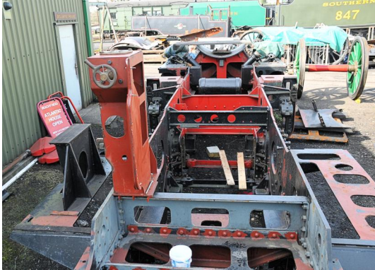
Driver's Pedestal trial fitted.
