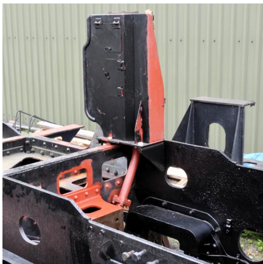
Driver's Pedestal with Train Pipe
