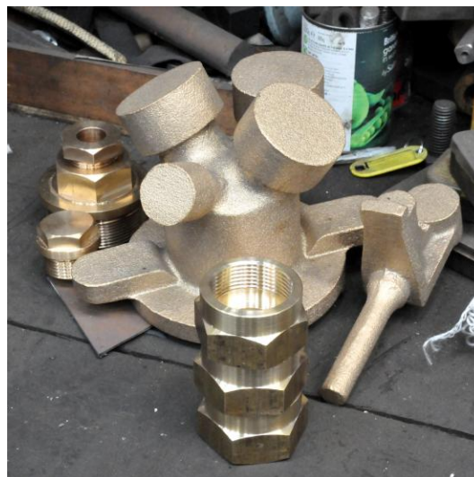
Sanding Valve and fittings
