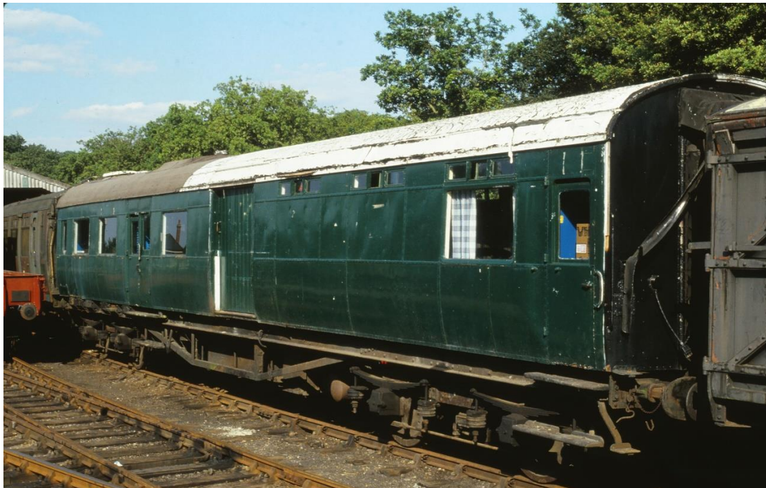
The west side of 7864 in 1982. The large sliding door in the middle of the coach is a Bluebell modification. Considerable further deterioration has occurred during storage since this image was taken. Photo: Tim Robbins
