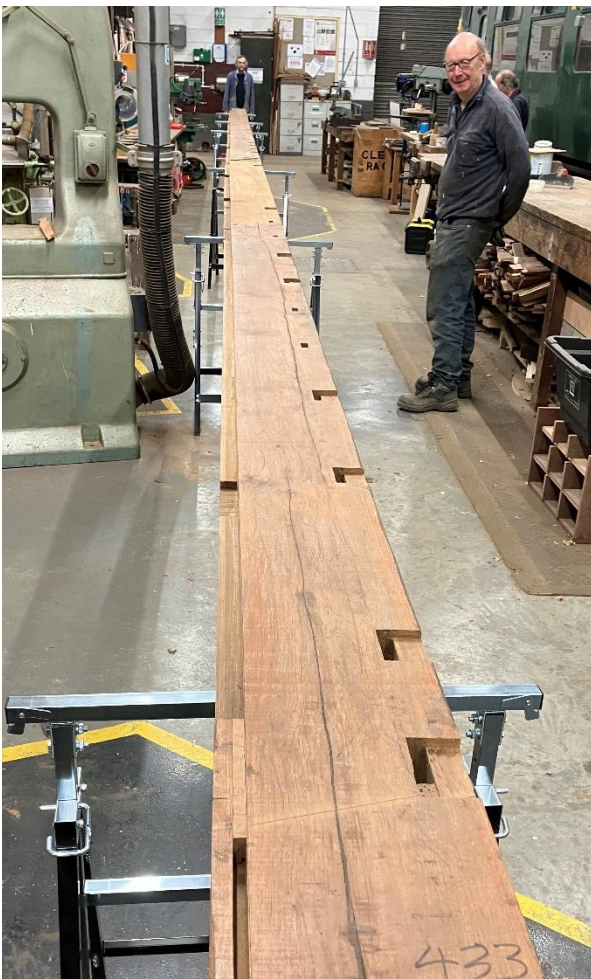
The four sections of the new west bottom side, set out and temporarily joined so that the chamfer could be applied to the front edge. May 2024
