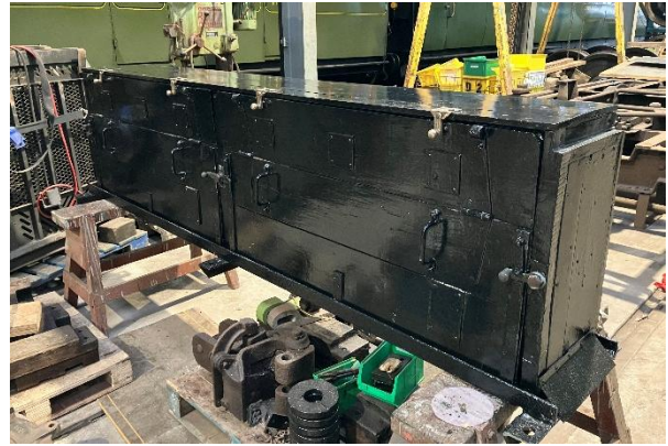
One of the two battery boxes, fully refurbished. It was fitted with a new top amongst other repairs. 6 Dec 2025
