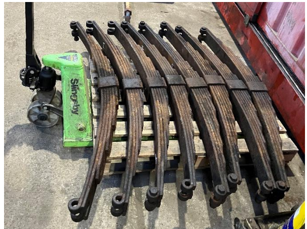
The eight leaf springs from 7864's bogies collected together on a sturdy pallet. 25 Feb 2026
