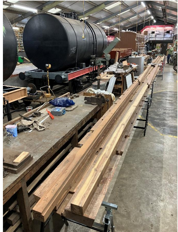
The east and west bottom sides and cantrail all laid out to check their alignment. 6 December 2025
